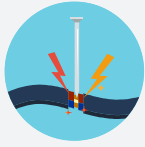
Wiring damaged by screws or nails
